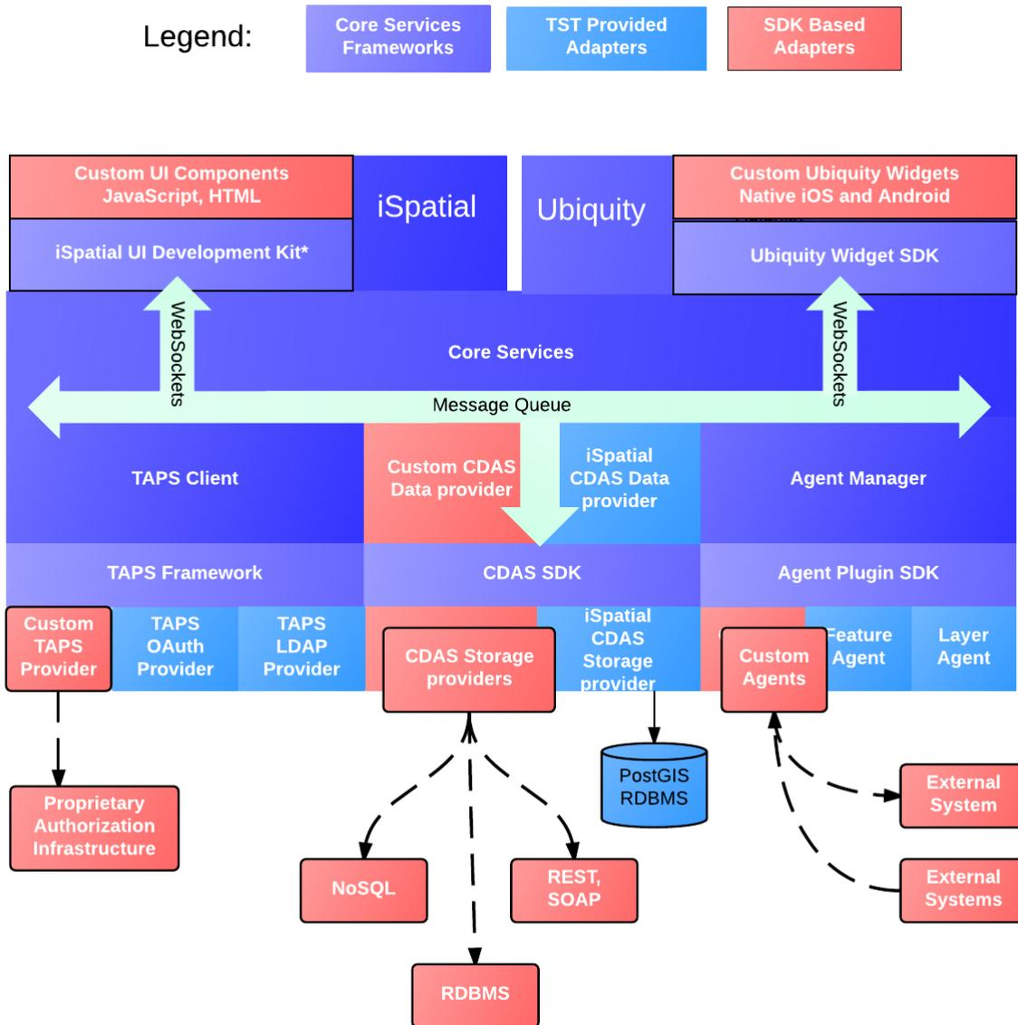
Figure 2 - iSpatial and Core Services and SDK Component Adapters
